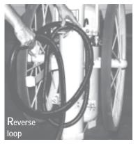
3. The next loop is a regular "hose in front" loop. Adjust the loops so that they are approximately the same size and then attach the hose to the shutoff valve with either the extension wand or nozzle installed.
